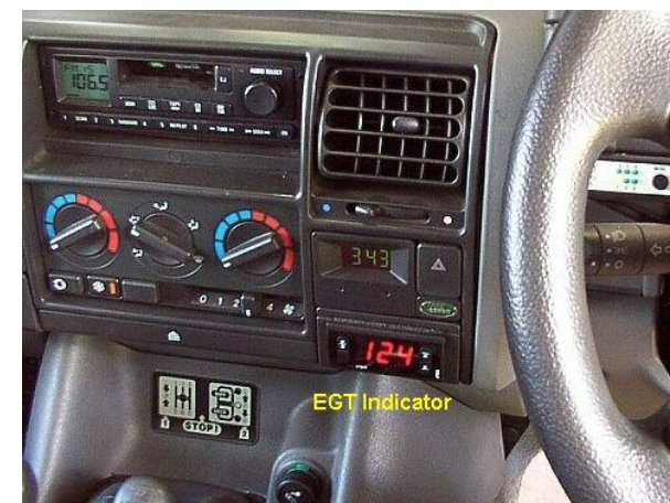
ThermoGuard Digital EGT Indicator with min/max recording function
