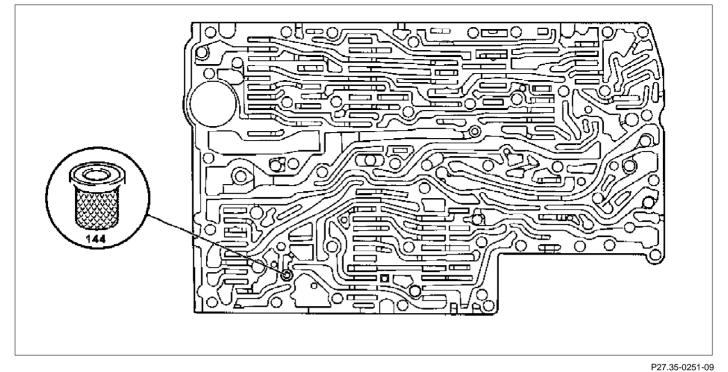
144 Strainer/converter lock-up control solenoid valve
