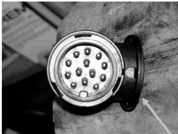
Male connector view MB Part # A601.540.11.81
