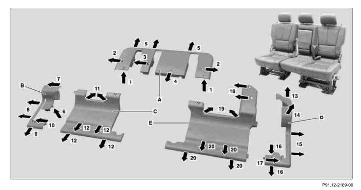
Arrows Pushing directions for releasing the locating tabs
