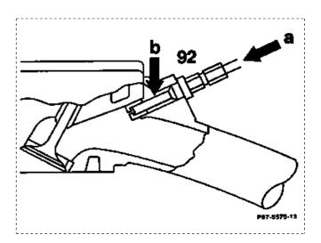
Air-enveloped injection valve Engines 103/104
