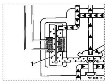
If the valve plate (1) is moved out of the middle position in the direction of fuel feed by a control current, the mixture is enriched.
