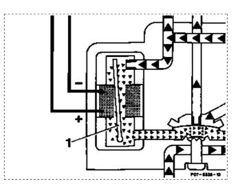
On vehicles fitted with catalytic converter and lambda control, the valve plate (1) constantly moves around its middle position in order to produce the necessary richer or leaner mixture. The KE control unit constantly alters the direction of the current for this purpose.
