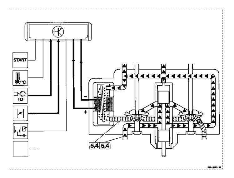
System pressure/upper chamber pressure Lower chamber pressure Injection pressure pressureless
