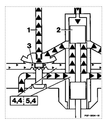
If the lower chamber pressure is high, this produces a lower pressure difference at the metering slots and thus a leaner mixture. Example for leaner mixture by means of electronic mixture adaptation (position of control piston (2) constant):
