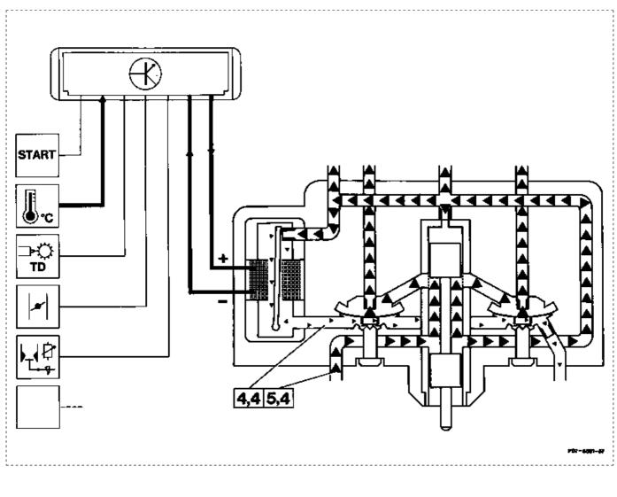
System pressure/upper chamber pressure Lower chamber pressure Injection pressure
