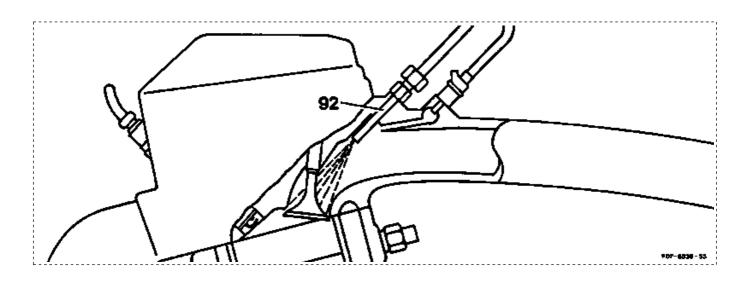
An injection valve (92) is positioned in the intake manifold for each cylinder of the engine. The injection valves spray the fuel metered by the fuel distributor continuously into the intake ports downstream of the injection valves. The injection valves do not perform any metering function.
