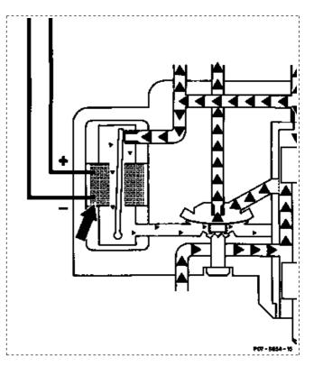
By altering the direction of the current at the solenoid, the valve plate is moved away from the fuel feed. The lower chamber pressure rises and the pressure difference at the metering slots is thus less.
