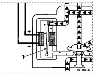
If the direction of the control current is altered, i. e. a change in polarity is performed at the solenoid, the valve plate (1) is moved out of the middle position toward the fuel feed. This produces a leaner mixture.
